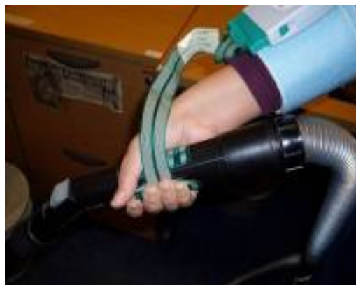
Figure 14: Thin Film Force sensor on vacuum handle
