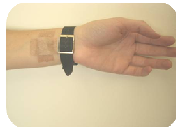
Figure 6: Fixation of a thermistor on the internal region of the wrist of the non-dominant hand with skin-colored tape.
