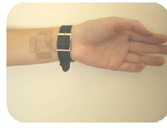
Figure 6: Fixation of a thermistor on the internal region of the wrist of the non-dominant hand with skin-colored tape.
