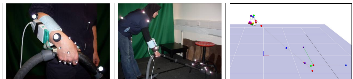
Figure 16: Close-up of had set-up for laboratory experiments, laboratory set-up for hoovering under a chair, motion capture analysis
