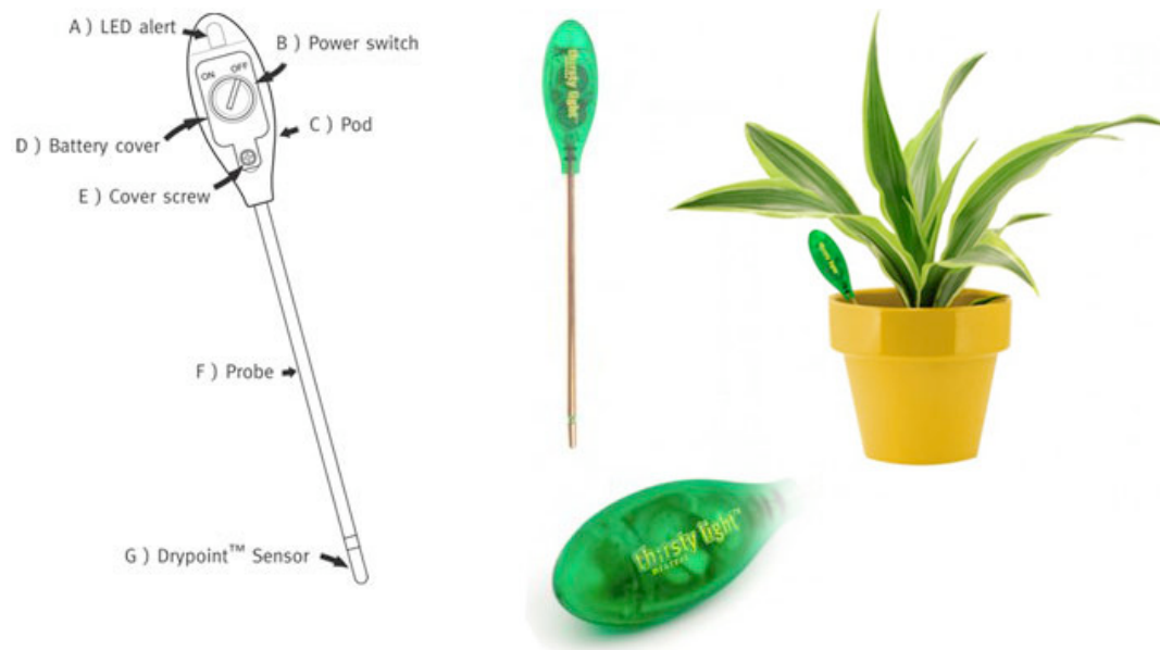
Figure 6: Thirsty Light, appliance designed to monitor the moisture of the soil and alert you when the plants need to be watered. ( http://www.thirstylight.com )
